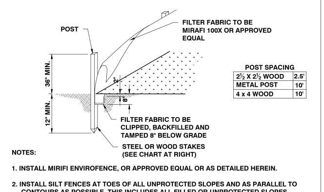
CONTOURS AS POSSIBLE. THIS INCLUDES ALL FILLED OR UNPROTECTED SLOPES CREATED DURING CONSTRUCTION. NOT NECESSARILY REFLECTED ON THE FINAL PLANS. CURVE THE ENDS OF THE FENCE UP INTO THE SLOPE. REMOVE SEDIMENT WHEN ACCUMULATED TO HALF THE HEIGHT OF THE FENCE. SILT FENCES ARE TO BE MAINTAINED UNTIL SLOPES ARE STABILIZED.
