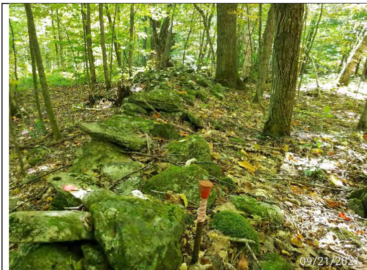
Photo 13 Subject: Stone wall and pin marking boundary
